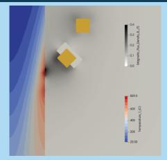
2D simulation of induction heating of shaft with scanning. **Magnetic field intensity** is shown in grayscale.
