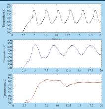
Temperature observed in simulation at the point on the surface of shaft. Different scanning velocity was used (from top to bottom) 10 mm/s, 6 mm/s 4 mm/s)
