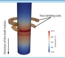
Numerical simulation was done with scanning of ø52 mm low carbon steel 1020 shaft. Used frequency 15 kHz, current 3600 A.
